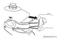
5. Tighten the three bolts (**A**, **B**, **C**) fastening the tank and one bolt (**D**) fastening the recoil starter.
