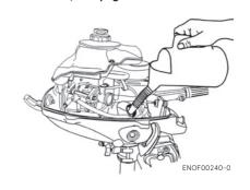
Use only high quality 4-stroke engine oil to insure performance and prolonged engine life.
