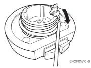
Tie a loop in the another end of the emergency starter rope and attach socket wrench that is included in the tool kit. 7
