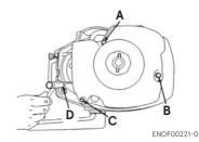
Insert the knotted end of the starter rope into the notch in the flywheel and wind the rope around the flywheel several turns clockwise.
