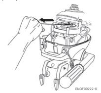
After engine starts, do not reinstall flywheel cover and top cowl.
