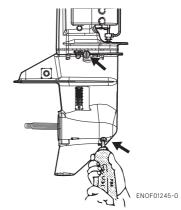
4. Install the upper oil plug, and then remove oil tube nozzle and install the lower oil plug.
