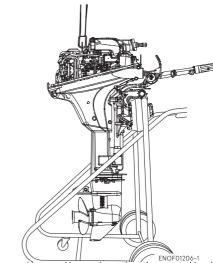
Keep the outboard motor in a vertical position when mounting.
