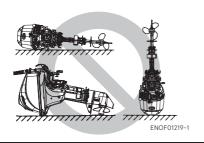
Keep the outboard motor in a vertical position when carrying.
