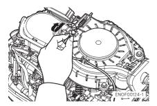
4. Remove the bolts (3pcs) and remove the recoil starter.
