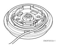
Tie a loop in the another end of the emergency starter rope and attach socket wrench that is included in the tool kit.
