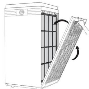
After replacing the filters, press the ⏻ and 🌙 buttons simultaneously for 3 seconds to reset the filters replacement indicator.
